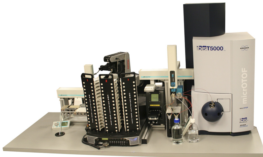
Figure 1. The Ibis T5000 universal biosensor. Shown in this view are key modules including amplicon purification and the mass spectrometer. Precise molecular weight determinations of amplicons yield unambiguous base compositions that are used to uniquely “fingerprint” each pathogen. The automated system is capable of analyzing over 1500 PCRs in 24 h.
